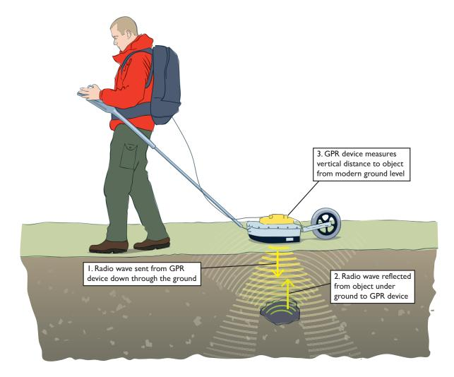
Fig. 2 How GPR works
